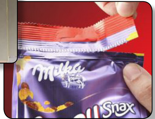
Packaging Scoring and Perforations with Lasers
