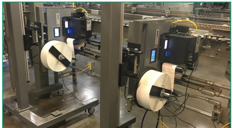
A pair of 255 systems in Zero Downtime configuration
